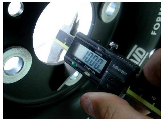
Formrace V4 – VALID (8 Small Ventilation Windows, with metallic inserts and 10mm thicker aluminum)
